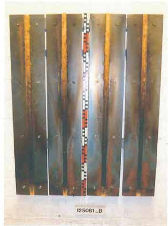
Figure 4: Appearance of specimen B after 10-minutes burning
