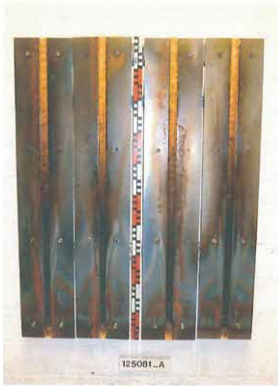
Figure 3: Appearance of specimen A after 10-minutes burning
