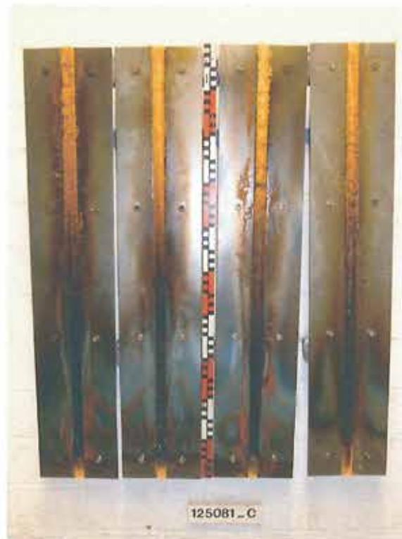
Figure 5: Appearance of specimen C after 10-minutes burning
